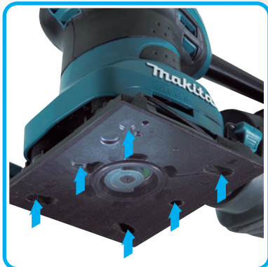
High Dust Extraction Dust is extracted through 6-hole under Pad and collected into Dust Bag. Also, instead of Dust Bag, Makita Vacuum Cleaner can be connected to the tool using Adapter.
