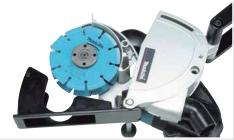
For blade change, simply loosen a bolt.
